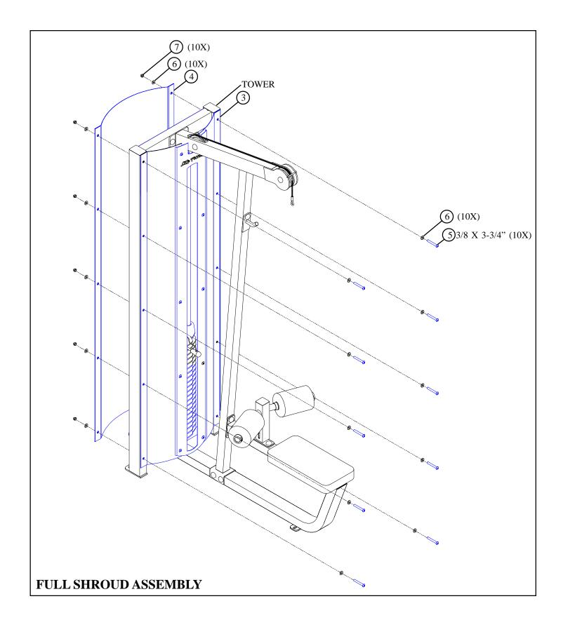
• **SECURELY** assemble the FRONT FULL SHROUD (3) and the REAR FULL SHROUD (4) to the TOWER using ten 3/8 X 3-3/4" BUTTON HEAD BOLTS (5), twenty 3/8" SAE BLK WASHERS (6) and ten 3/8" ACORN NUTS (7) as shown above.
